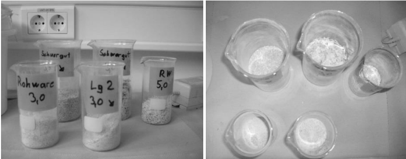
Figure 14. Fine ground GRP Source: HOBAS
