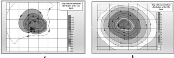
Fig. 3.Curves of isoconcentration for CO<sub>2</sub> (a) and CH<sub>4</sub> (b) in the ambient air
