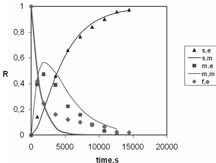
Fig. 3 – The variation of reduced concentrations of indole-3-acetic acid (IAA) in time. Experimental conditions: feed phase: indole-3-acetic acid  $10^{-4}$  mol/L, membrane: solution of tributyl phosphate  $10^{-2}$  mol/L in chloroform, stripping phase:  $10^{-2}$  mol/L NaOH solution, transport time 4 hours, stirring speed: 180 rot/min.
