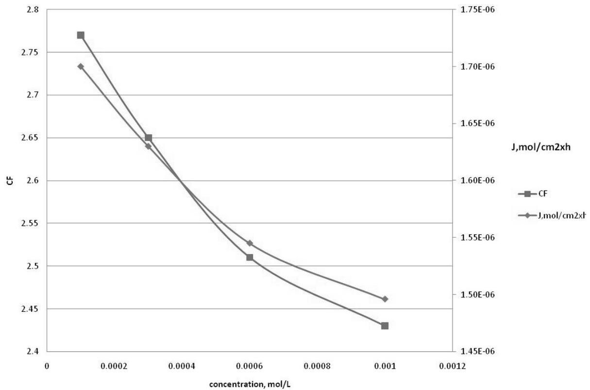
Fig. 1 – The effect of indole-3-acetic acid (IAA) concentration from the feed phase on the flux ( $J$ ) and the concentration factor (CF). Experimental conditions: feed phase: indole-3-acetic acid  $10^{-4} - 10^{-3}$  mol/L, membrane: solution of tributyl phosphate  $10^{-2}$  mol/L in chloroform, stripping phase:  $10^{-2}$  mol/L NaOH solution, transport time 4 hours, stirring speed: 180 rot/min.
