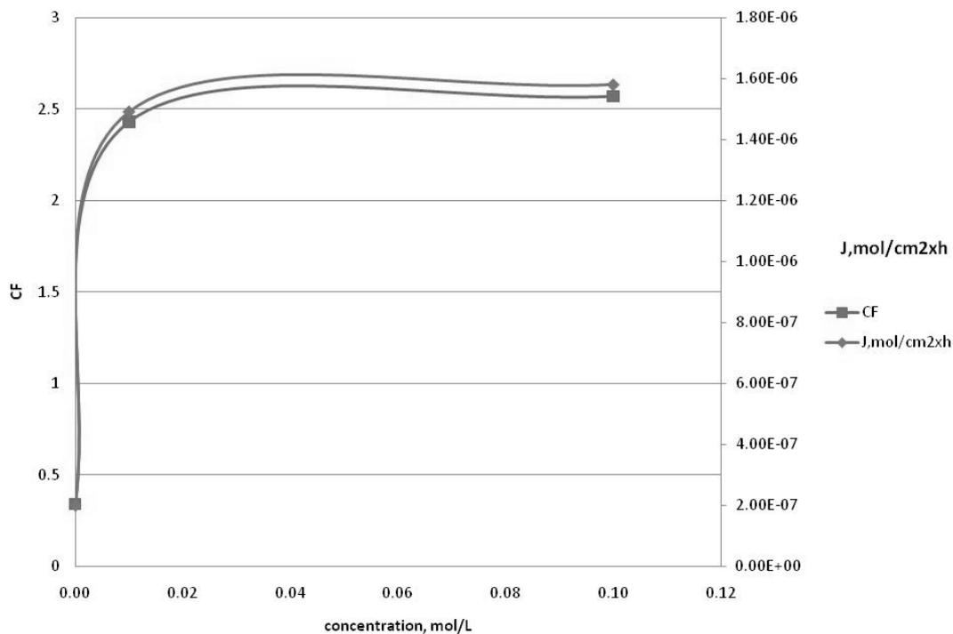
Fig. 2 – The effect of sodium hydroxide (NaOH) concentration from the stripping phase the average flux ( $J$ ) and the concentration factor (CF). Experimental conditions: feed phase: indole-3-acetic acid  $3 \times 10^{-4}$  mol/L, membrane: solution of tributyl phosphate  $10^{-2}$  mol/L in chloroform, stripping phase:  $10^{-2} - 10^{-1}$  mol/L NaOH solution, transport time 4 hours, stirring speed: 180 rot/min.
