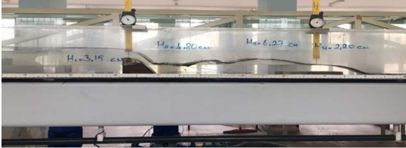
Figure 3. Water surface profiles at model
