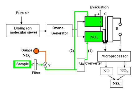
Figure 1 Schematic representation for utilization of the luminescence method for monitoring of the NO<sub>x</sub> from air
