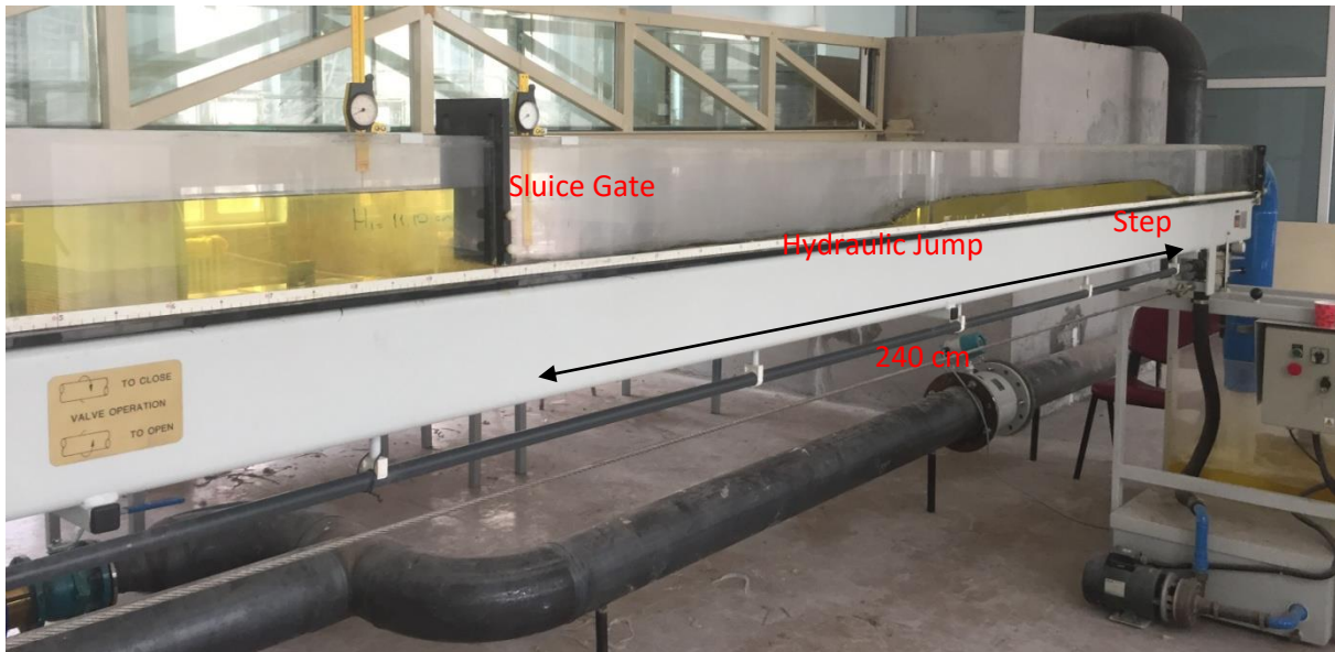
Fig. 6. General view of the open channel system
