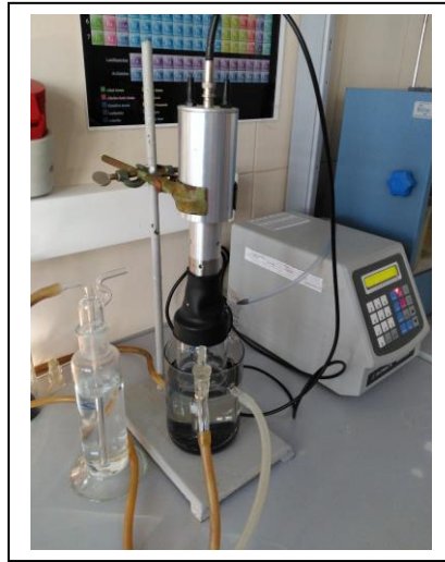
Fig. 1. Ultrasonic reactor - closed system
