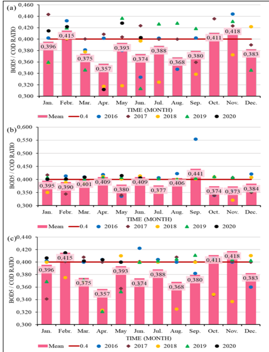
Fig. 2. Variation of the ratio BOD 5 /COD monthly for wastewater samples in three station: IS (a), SV1 (b) and SV2 (c), 2016 ÷ 2020
