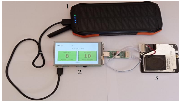
Fig. 2. Photo of the set-up used for the air analysis: 1- Solar battery (WBPINE Model N° F16SL), 2-data logger (KCEMC1 1728-94V-OF1-H4) with display (3.5inch RPi Display), and 3-PM2.5 and PM10 sensor (nova PM sensor, type SDS011) with USB stick (USB2TT-004)
