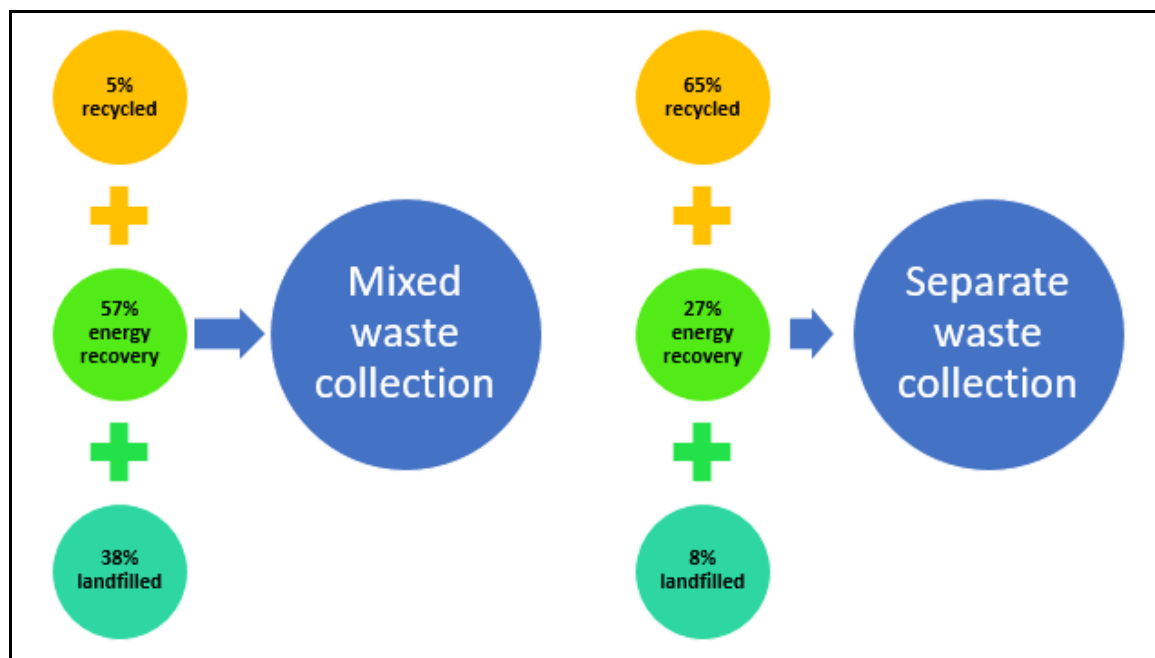
Fig. 2. The percentage of recycled plastic for separate waste collection versus mixed waste collection
