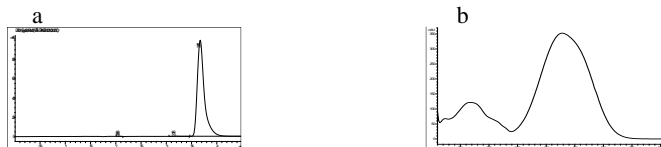
Fig. 1. HPLC chromatogram obtained for 10 mg/L MO (a); The UV-VIS spectrum registered for the MO dye (b).
