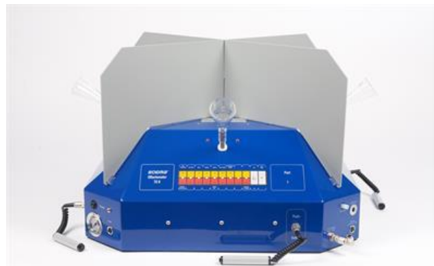
Fig. 3. Dynamic olfactometer with 4 positions Olfasense TO8 used to determine odour concentration [6]
