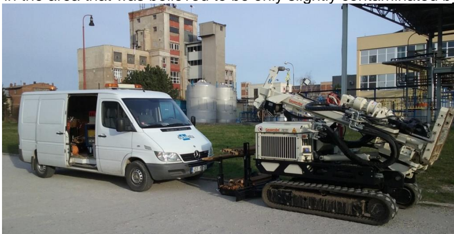
Figure 2: Geoprobe rig 7822DT and MIP van on the Moravian site
