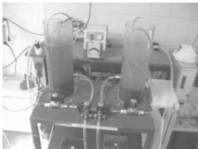
Fig. 1. Sequential bioreactors pilot laboratory installation
