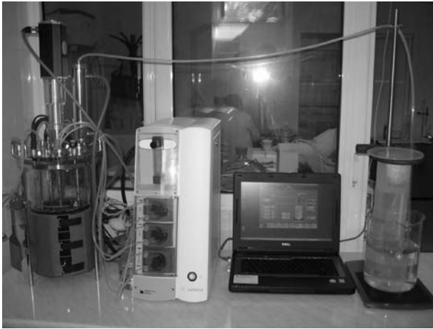
Fig. 1. Experimental setup for biogas production
