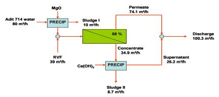
Figure 2 Flow sheet of membrane test work for a specific blending ratio of ARD and Rosia Valley flow
