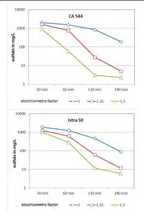
**Figure 1** Residual sulphate concentration in the supernatant in dependence of reaction time and stoichiometric excess for ettringite precipitation using Wahalla lime (CA S44) and Istra 50
