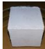
Fig.3. Aspect of concrete sample containing the WEEE polyamides
