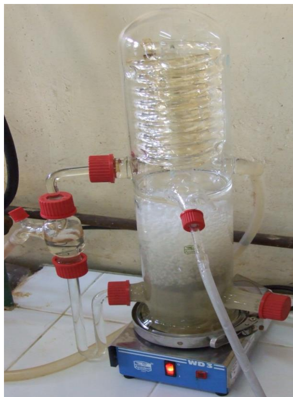
Desktop distilled water apparatus ASSISTANT 225
