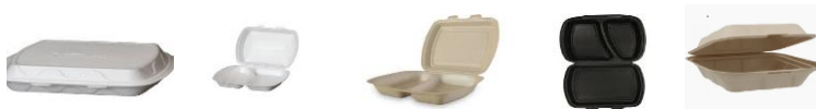
Figure 1. Samples from extruded polypropylene, extruded polystyrene (white, cream, black) casseroles, sugar cane fiber.
