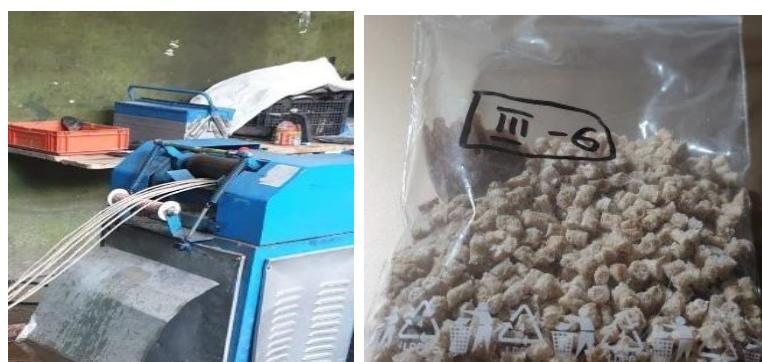
Figure 2. Single screw extrusion process and resulting composite pellets.
