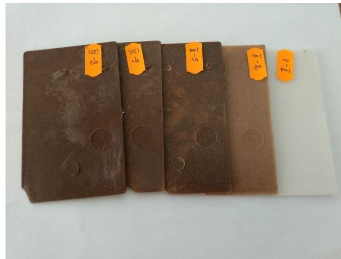
Figure 4. Composites sample prepared using injection molding process (I-LDPER; II-LDPER/10FF; II-LDPER/20FF; II-LDPER/30FF; II-LDPER/50FF).
