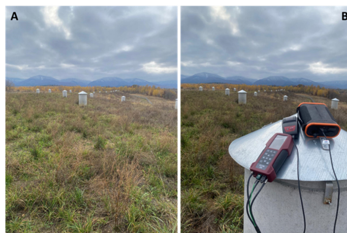
Figure 4. Images from the site of a municipal solid waste storage station (A); the measurement of \text{CH}_4 and \text{CO}_2 from the biogas capture well (B).
