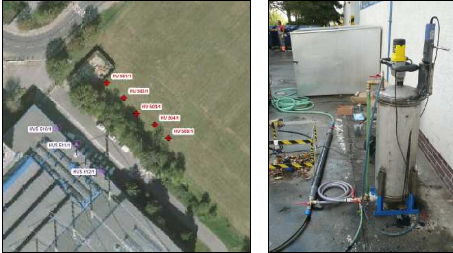
Fig. 4: nZVI pilot-scale set up (left – wells' layout; right – an injection device)
