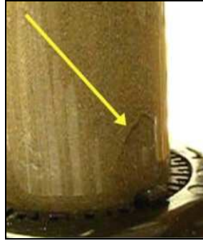
Fig. 9: The self-mixed pocket causing formation of a preferential way
