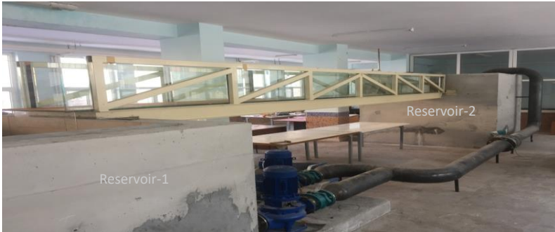
Figure 3. Open channel system used in experiments
