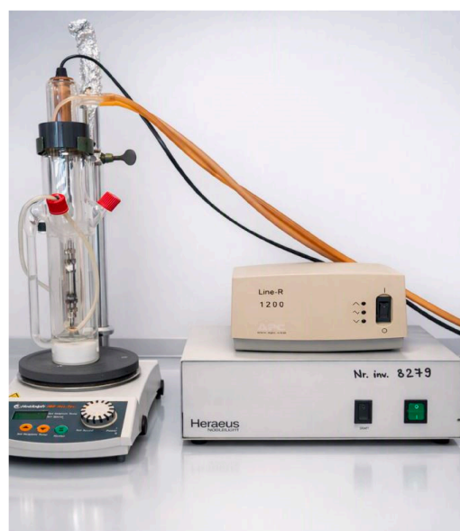
Figure 9. Experimental photocatalytic reactor setup.
